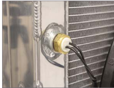
Built in temperature sender boss
